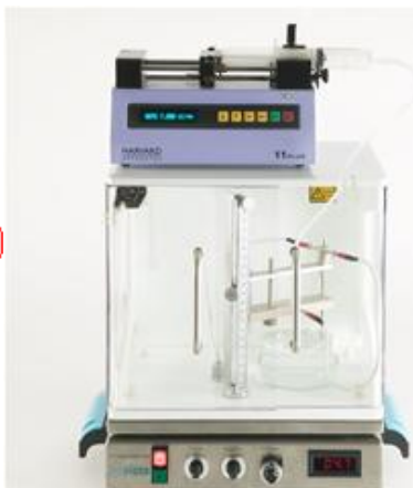
Var V1 (Nisco, CH) - electrostatic capsule generator
